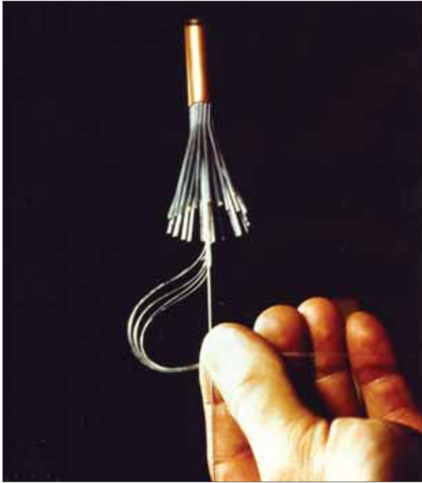
Figure 1.7: A section of TAT-8, the first trans-oceanic fibre-optic cable which, together with a developing internet, heralded a new age of communications. Source: AT&T Inc.
