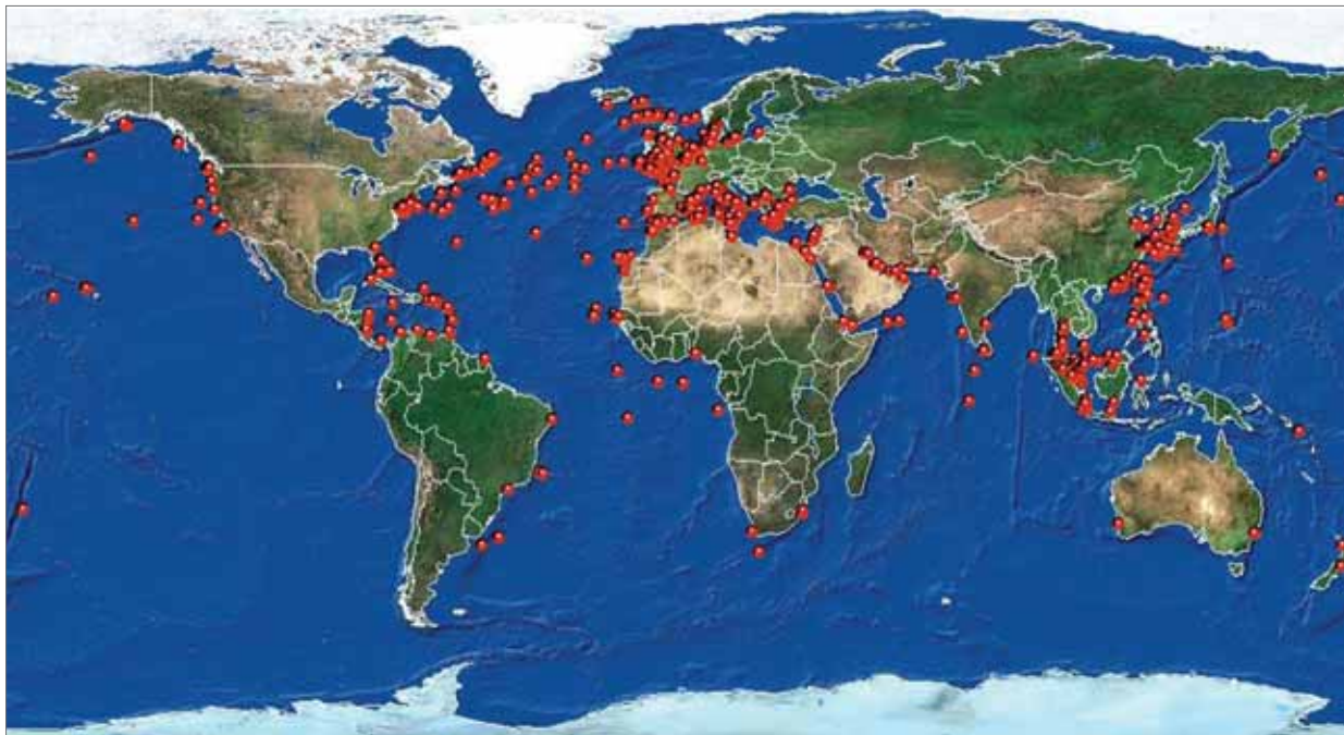
Figure 7.3: Global pattern of external aggression cable faults, 1959–2006. Source: Tyco Telecommunications (US) Inc.
