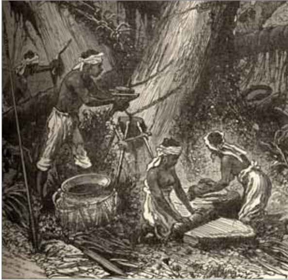
Figure 1.1: Tapping gutta percha, a natural polymer used for insulating early submarine cables. Source: Bright (1898); courtesy of archives of BT Heritage.
