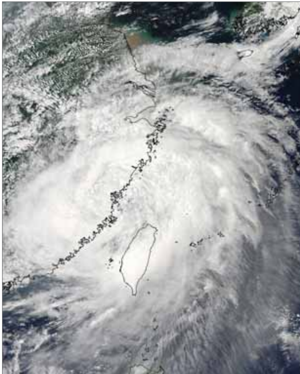
Figure 6.5: Typhoon Morakot struck Taiwan over 5–11 August 2009, when 3 m of rain fell in the central mountains, causing rivers to flood and carry large volumes of sediment to the ocean. So much sediment was discharged that several submarine landslides and associated sediment-laden ‘turbidity currents’ formed and broke a succession of cables off eastern and southern Taiwan as well as the nearby Philippines. While records of such events are insufficient to identify trends, the enhanced precipitation of Typhoon Morakot is consistent with warmer regional air and ocean temperatures. Source: MODIS Rapid Response, NOAA.
