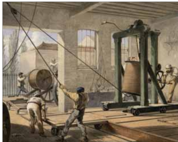
Figure 1.3: Loading gutta percha insulated cable for the Great Eastern cable ship. Source: courtesy of archives of BT Heritage.
