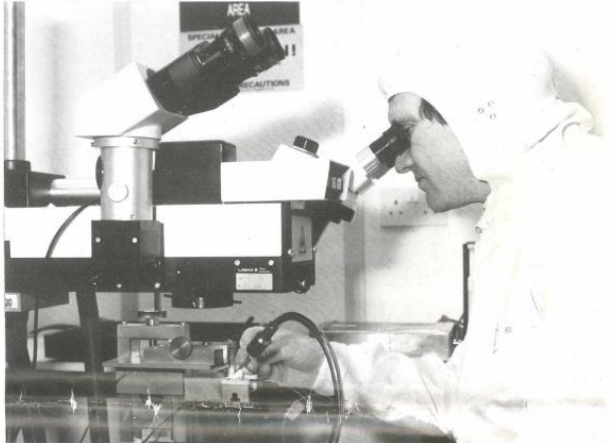
A laser welder being used in TA5.2.1 to assemble receivers for TAT8, the first transatlantic optical cable system.
