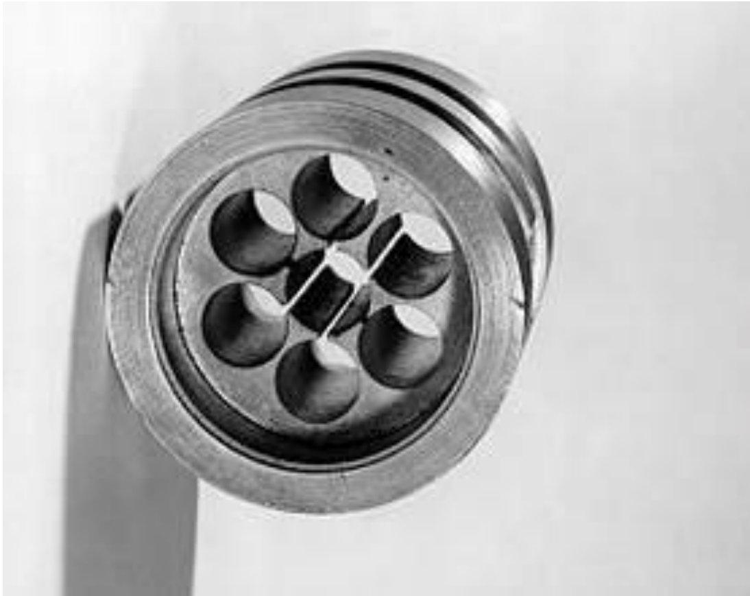
The anode block of an early cavity magnetron showing the initial 6 & later 8 cavity resonators
