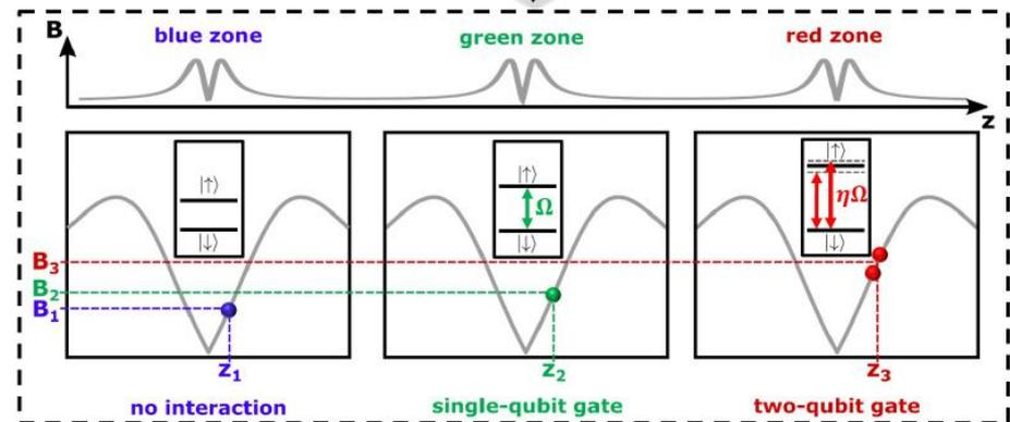
Voltages applied to local trap electrodes place the ion in the correct part of the local B-field gradient making the ion resonant with a set of global radiation fields, effectively executing a particular quantum gate.
