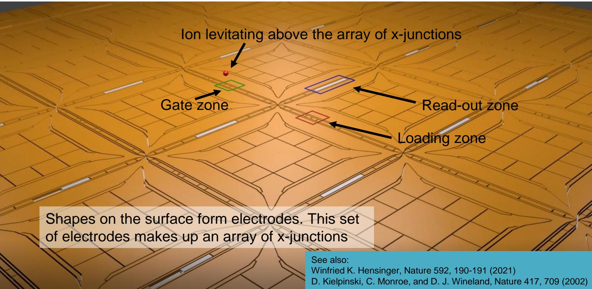
Ion levitating above the array of x-junctions
