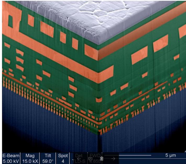
IBM microprocessor chip:
