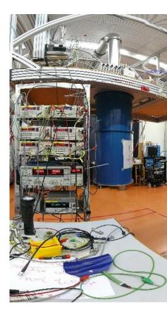
Dilution refrigerator in Andreas Wallraff's superconducting qubit laboratory at ETH Zurich
