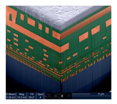
IBM microprocessor chip: Layer of transistors connected via multiple layers of wiring
