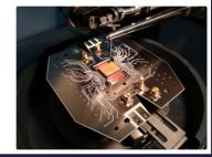
Legato: Prototype trapped ion quantum computer with four interconnected modules
