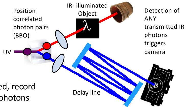
Illuminate object in the infra-red, record image using correlated visible photons
