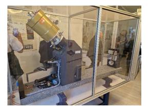
It was fascinating to learn how the spectrographs were used to detect 'wobbles' in a star's velocity in respect to the earth caused by planets orbiting it. While the earlier equipment was sensitive enough to detect changes in the ~100m/s range. This could detect large planets orbiting close to the stars termed hot-Jupiters. The newest equipment can detect 'walking speed' changes in velocity allowing for smaller and further away planets to be detected.
