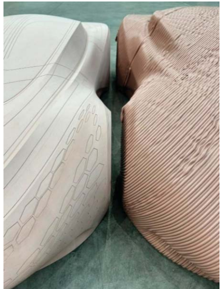
Full model printed vs milled
