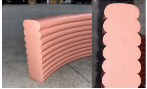
A printed part cut up, showing the fully dense layers
