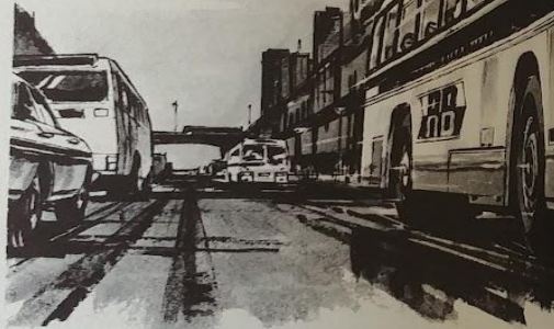
Above: Guided by a simple underground cable, a driverless bus heads down a busy high street.
