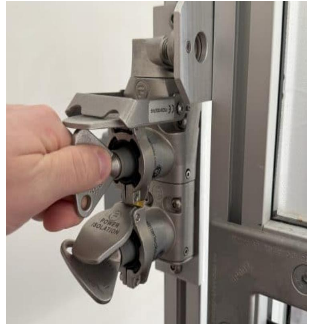
Figure 2.14 Fortress Double lock gate access system
