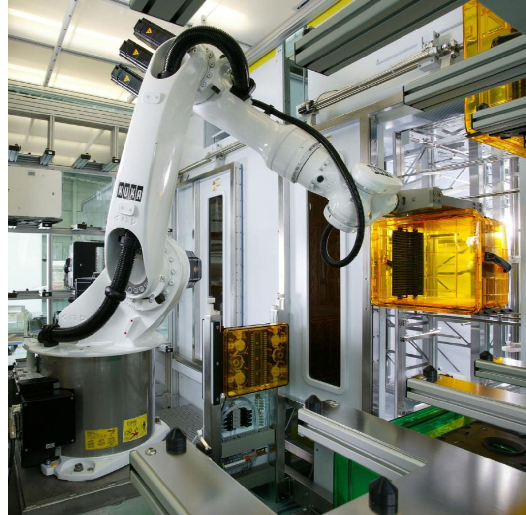
Figure 2.29 Kuka Robot in SemiConductor wafer fabrication
