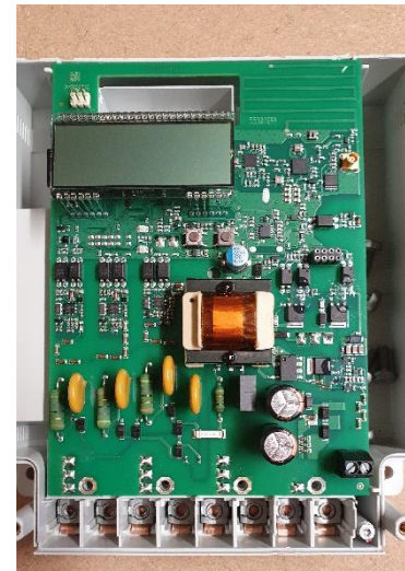
Smart meter with built-in power supply and processor capacity that creates more voltage noise while having less efficient noise filters.
