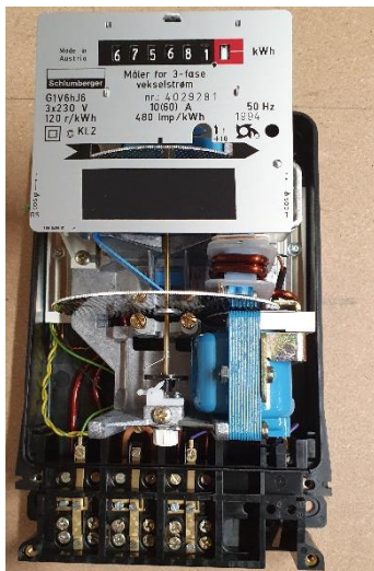
Analogue mechanical meter with rotary dial, without built-in power supply.
