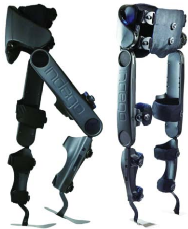
The Indego is a robotic exoskeleton designed to help patients with lower limb paralysis walk again. During development, Parker Hannifin used Protolabs to quickly test design improvements.
