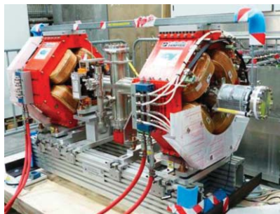
A LINAC Warm Unit (LWU) for the European Spallation Source (ESS) in Lund, Sweden. This will be the world's most powerful Neutron Source. Credit STFC
