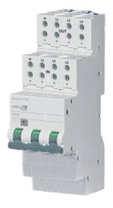
Triple pole RCCB with switched neutral. For adding RCD protection to an MCB or HBC fuse on 3-phase or split-phase outgoing circuits. 100A rated for general application. All units are three modules wide.
